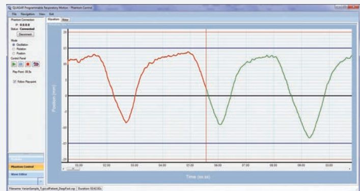
Above: Screenshot of the QUASAR TM Respiratory Motion Software, featuring the Phantom Control module.
