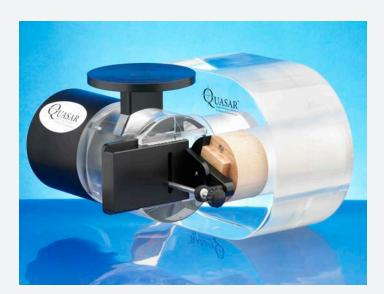
**Above:** The QUASAR Respiratory Motion Phantom with Rotation Stage enables cylindrical inserts to rotate as they translate with a 60° total range of motion (± 30° from the horizontal).
