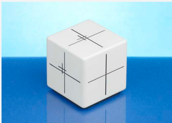
Above: The acrylic 5 x 5 x 5 cm QUASAR™ IsoCenter Cube Phantom used for measuring isocenter accuracy
