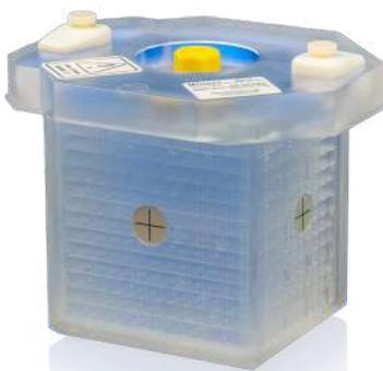
Above: The QUASAR GRID<sup>3D</sup> acrylic cube containing a 1cm<sup>3</sup> 3D grid of 1.5 mm channels filled with CuSO<sub>4</sub> solution.
