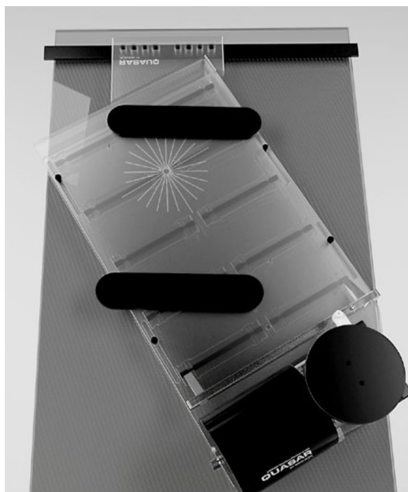
Above: Added IGRT gating QA onto Multi-Purpose Body Phantom
